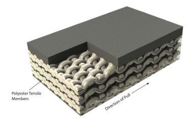
(Above) Our belts are constructed of polyester or nylon fabrics. Tough polyester filament yarns give GRT belts high tensile strength. The longitudinal warp yarns carry the tension, and the transverse fill yarns hold the wrap in place and retain the mechanical fasteners. The crimp in the fabric acts as a shock absorber, permitting the fabric to deflect and adjust itself during impact shock.
